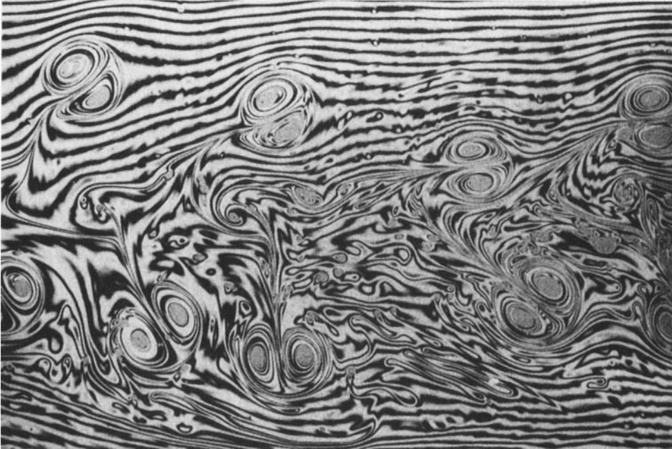
FIGURE 7. The cloud of couples created in a turbulent wake with f_m = 1.1 f_{ST} .
