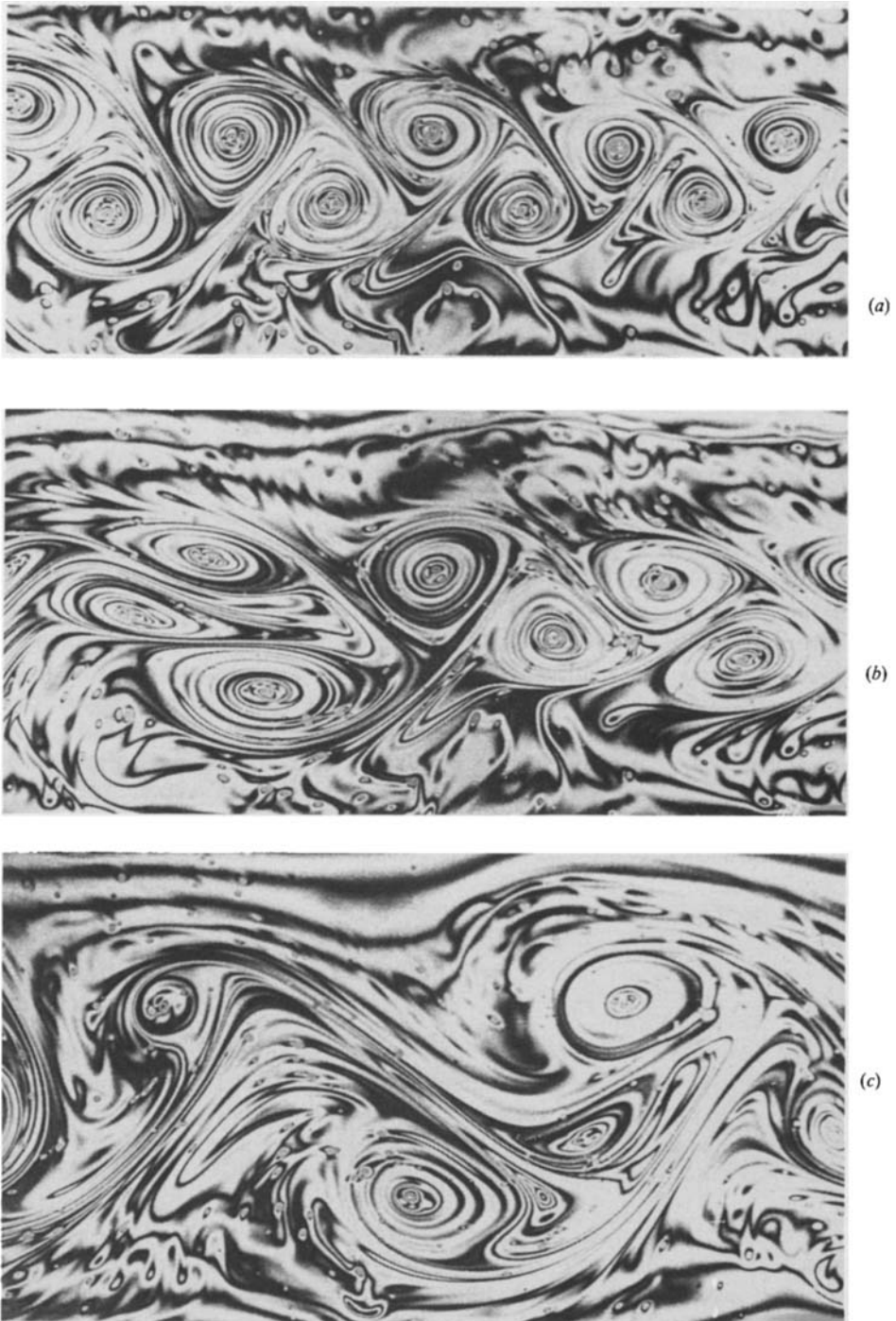
FIGURE 2. Three successive (in time) photographs showing vortices merging in a turbulent wake.
